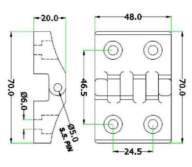
APPLICATION DRAWING FOR MODEL NO. KP 20.2 S/S (NYLON SHOE HINGE)
